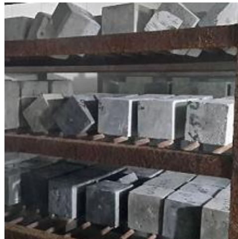
(c) 拆模后的试块养护
